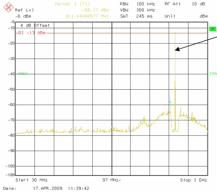
Fundamental test with band stop filter
