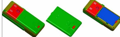
1. Follow the following steps for installation: 1. Insert upside of the battery in to holder . 2. push the bottom of
