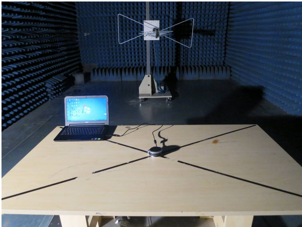
FCC RADIATED EMISSION TEST SETUP
