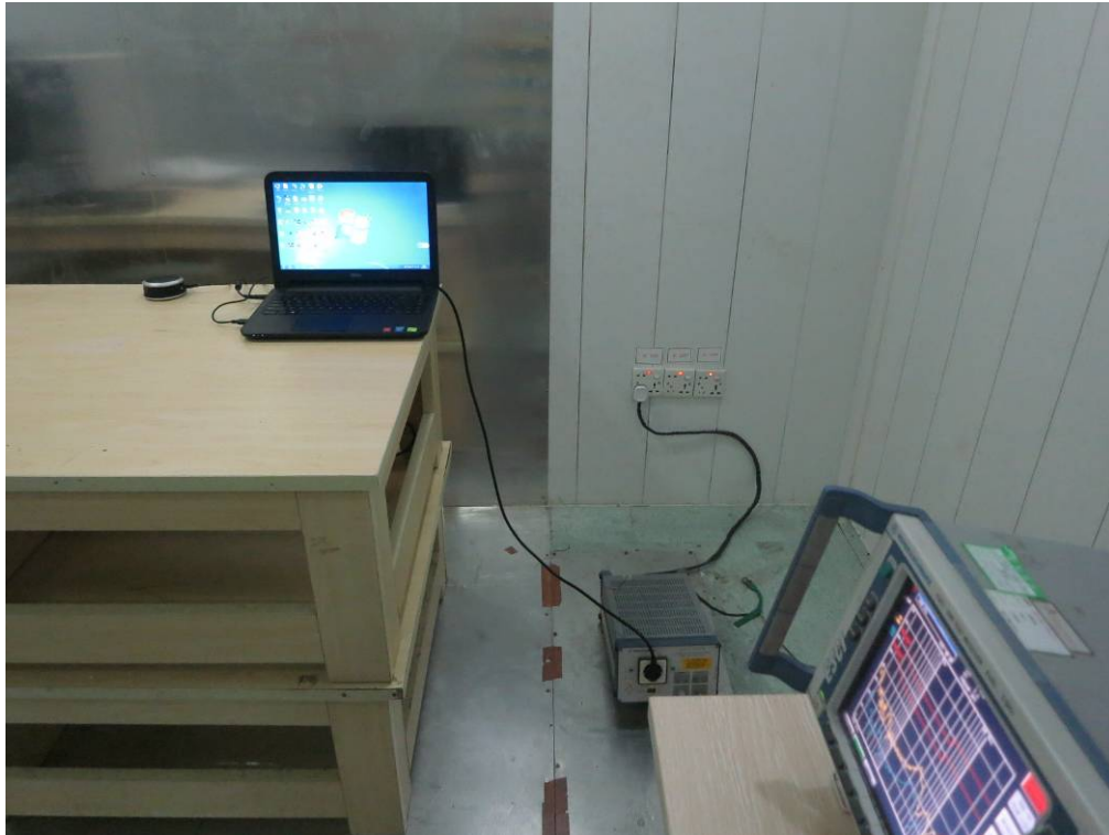
FCC RADIATED EMISSION TEST SETUP
