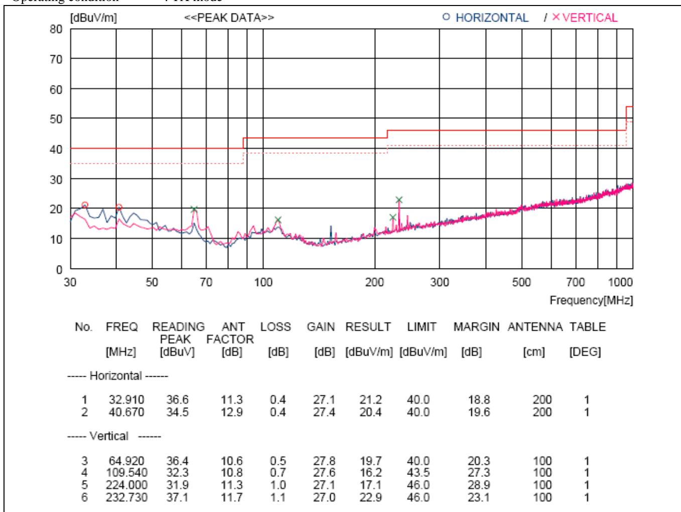
Remark: Margin (dB) = Limit – Result and Result = Reading Peak + Antenna Factor + Loss - Gain
