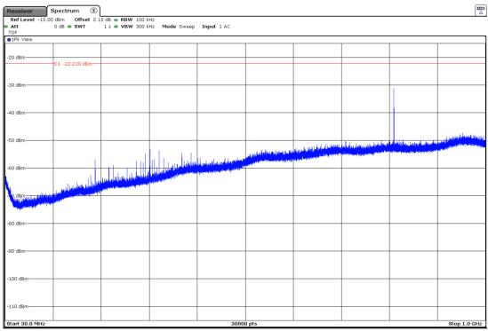
Note: The highest peak shown in the plot is the carrier frequency. The FCC limit set in -13 dBm lies above the Reference Level, thus outside the plot vertical scale. Compliance with the FCC limit is ensured, as the equipment meets the more-restrictive ISED requirement set in -22.23 dBm.
