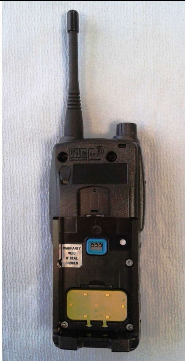
HTT-500-2 Rear View with battery removed
