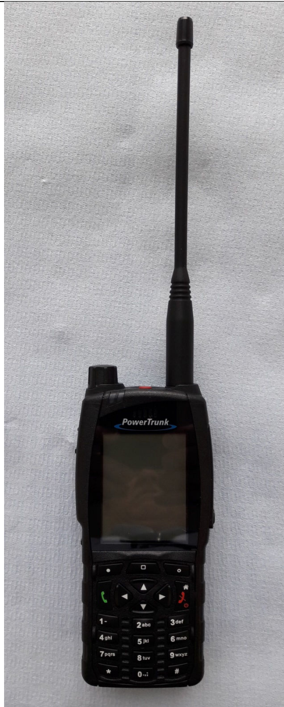
HTT-500-2 Front View fitted with ½ wave whip antenna
