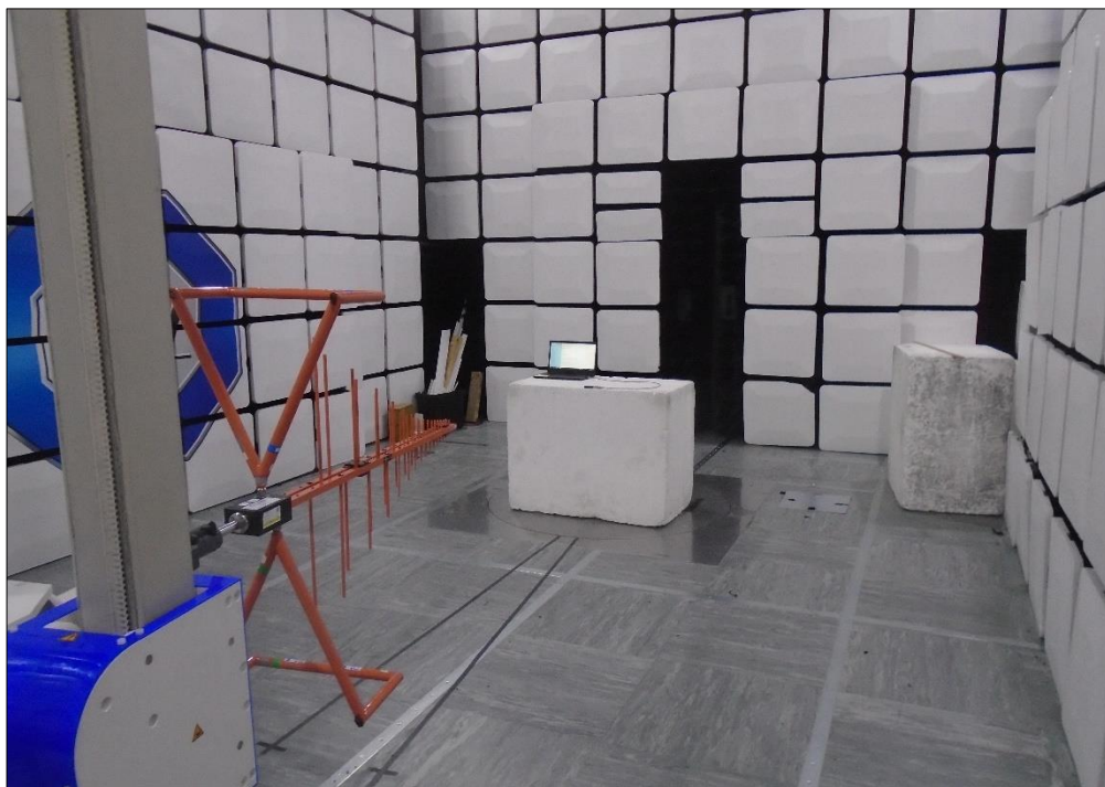
Figure 16 - Test Setup - 30 MHz to 1 GHz
