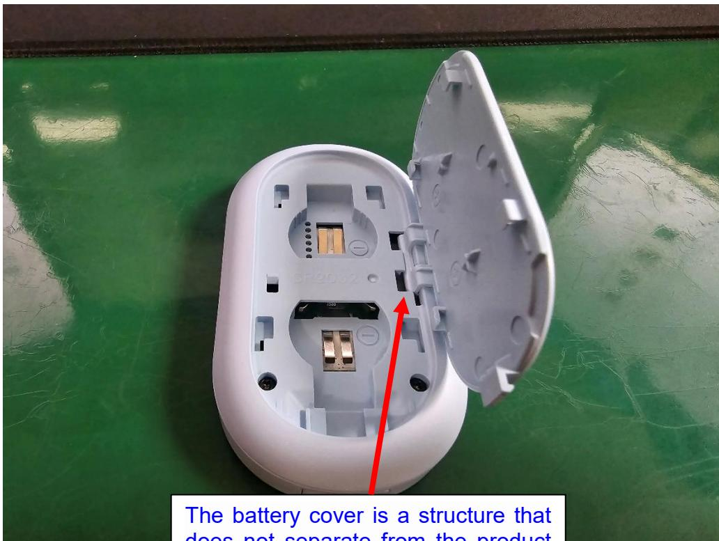
The battery cover is a structure that does not separate from the product body, and the label is attached to the battery cover corresponding to the rear of the product.
