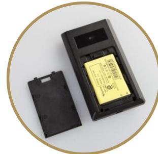
If keypad could not be charged normally, please replace the battery.
