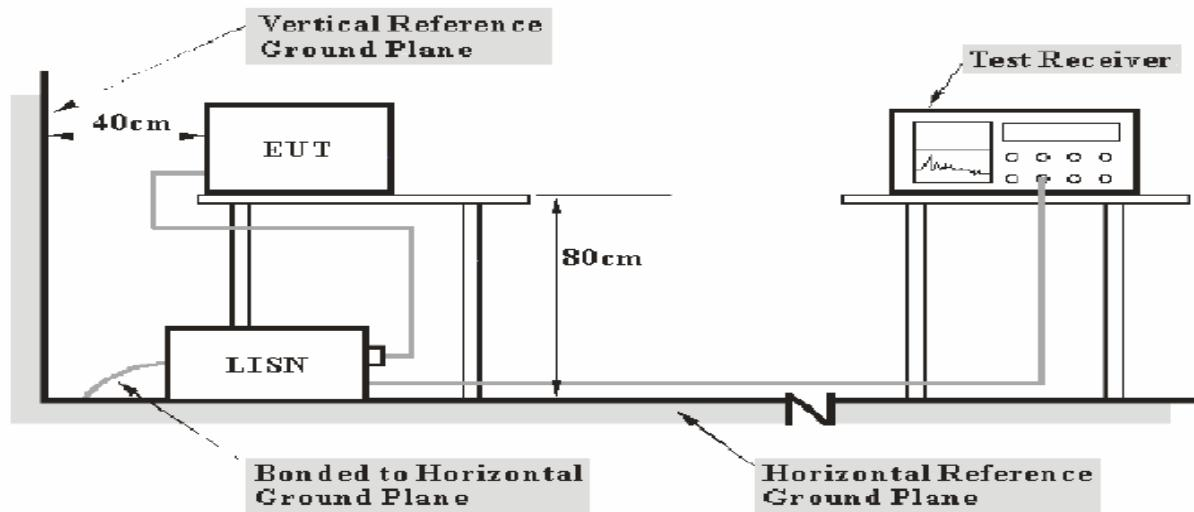
The setup of EUT is according with MP-5 measurement procedure. The specification used was the FCC Part 18 limits.
