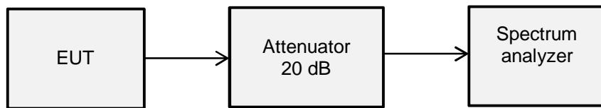
The EUT is set to transmit continuously at maximum RF power.
