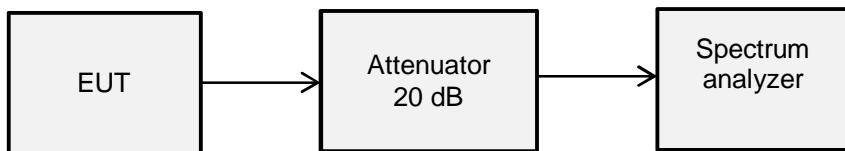
The EUT is set to transmit continuously.
