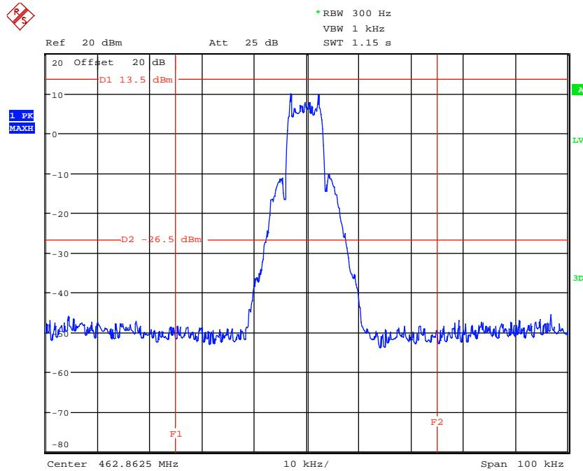
161191\_MID\_BURST.wmf: Spectrum mask, transmitter operates with burst modulation at 462.8625 MHz:
