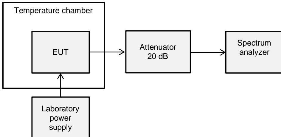
The battery of the EUT was removed. The EUT was supplied by a laboratory power supply.
