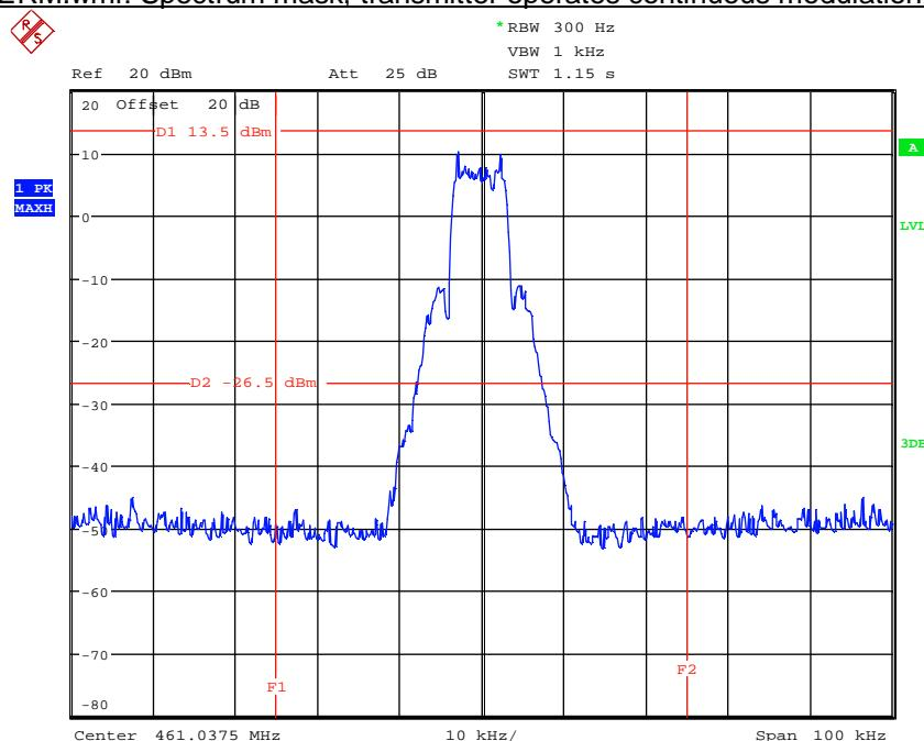
161191\_LOW\_BURST.wmf: Spectrum mask, transmitter operates with burst modulation at 461.0375 MHz:
