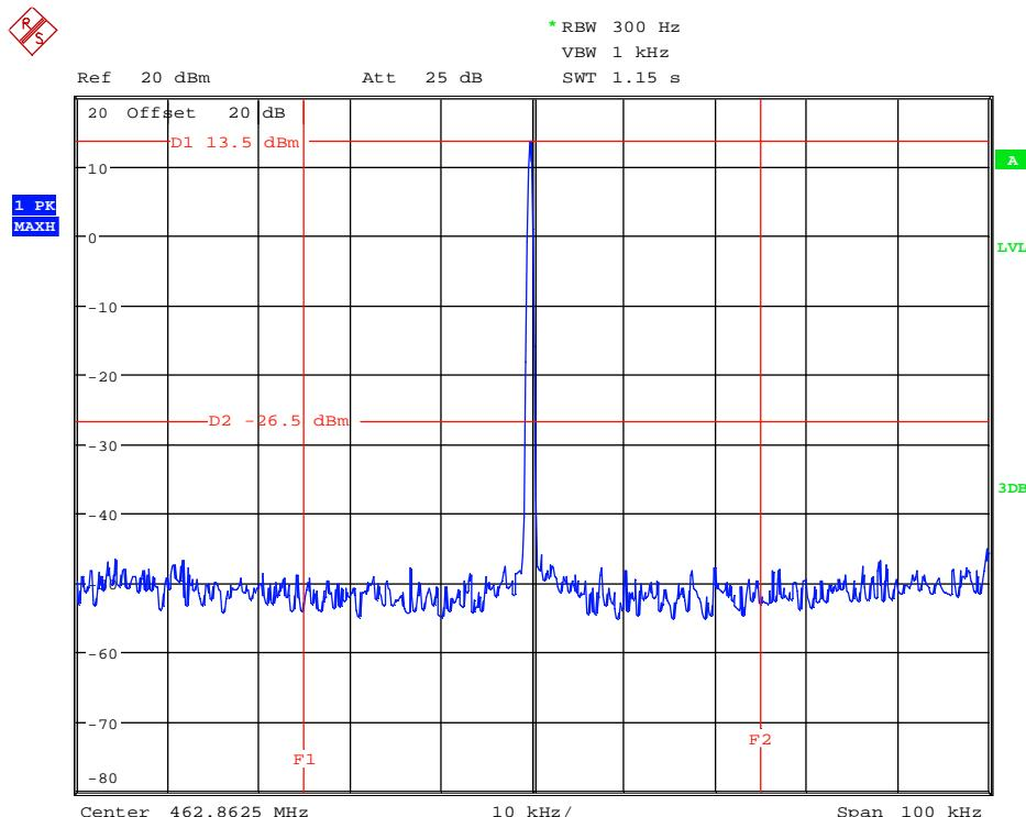
161191\_MID\_PERM.wmf: Spectrum mask, transmitter operates continuous modulation at 462.8625 MHz:
