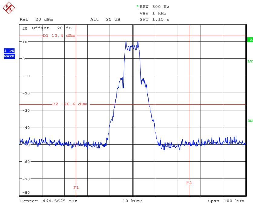
161191\_HIGH\_BURST.wmf: Spectrum mask, transmitter operates with burst modulation at 464.5625 MHz:
