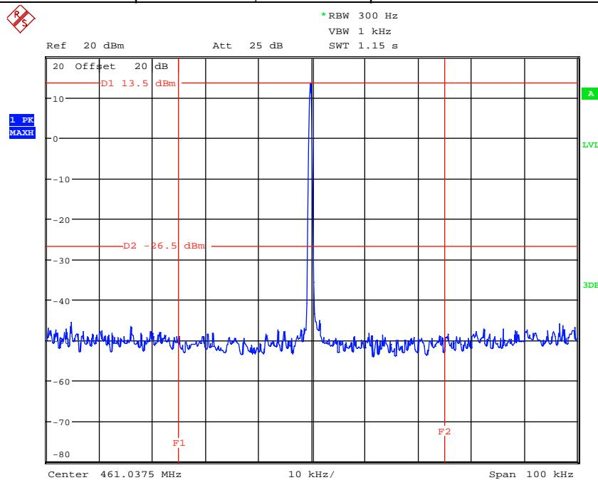
161191\_LOW\_PERM.wmf: Spectrum mask, transmitter operates continuous modulation at 461.0375 MHz:
