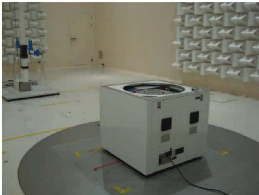
Setup Photo (Field Strength of the Fundamental Emission)
