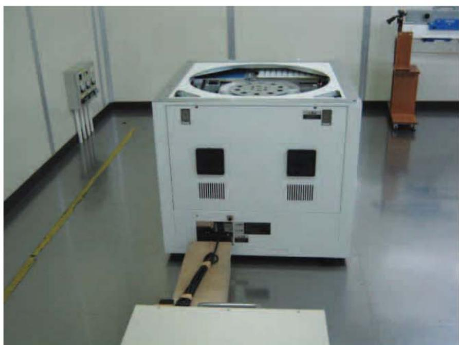
Setup Photo (Radiated Spurious Emission)
