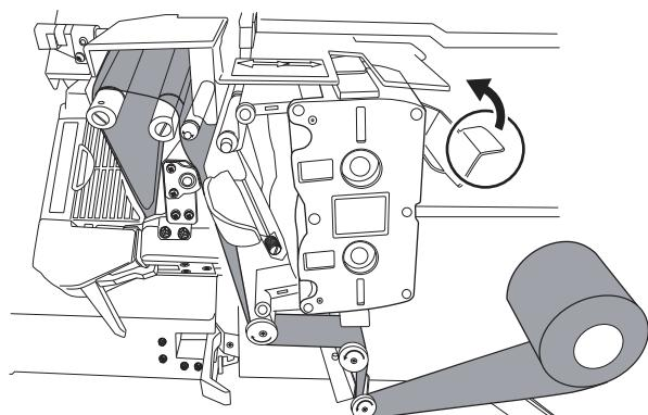
6. Return the printer head open lever to the original position.
