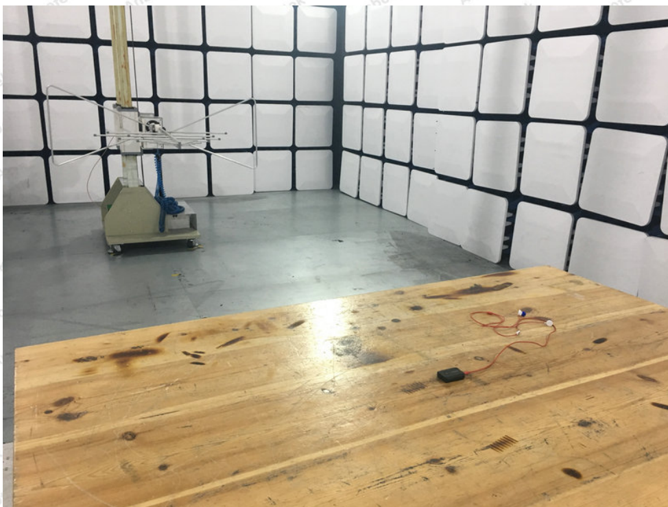
Photo of Radiation Emission Test
