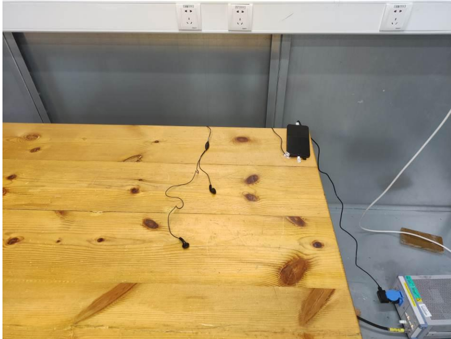
17. Conducted Emission (Part 15C, Wi-Fi/Bluetooth)
