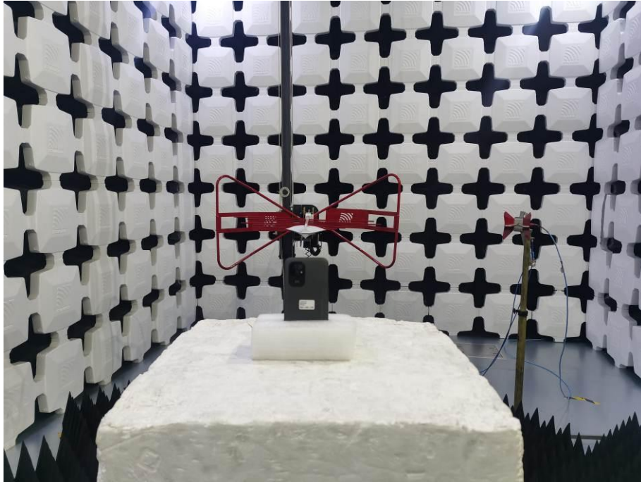
11. Radiated Emissions (Part 22/24/27,30MHz-18GHz)
