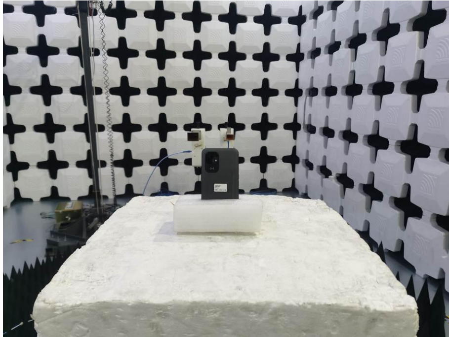
13. Radiated Emissions (Part 22/24/27, 26.5GHz-40GHz)
