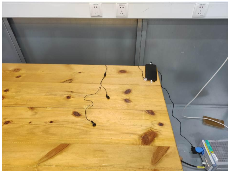
14. Conducted Emission (Part 15B, Camera/Video Player/FM receiver)
