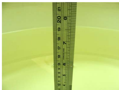
Fig 6.2 Photo of Liquid Height for Body SAR
