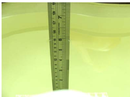
Fig 6.1 Photo of Liquid Height for Head SAR
