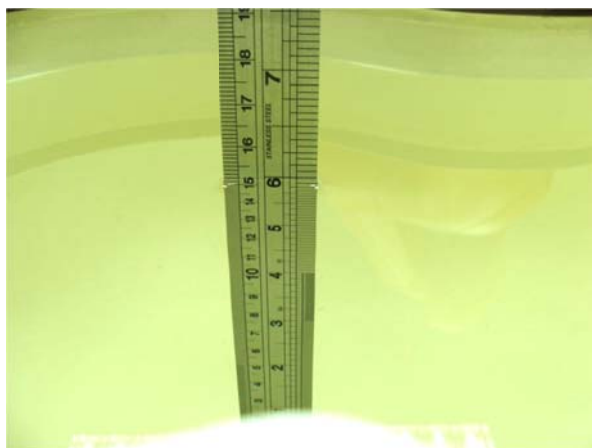
Fig 6.1 Photo of Liquid Height for Head SAR
