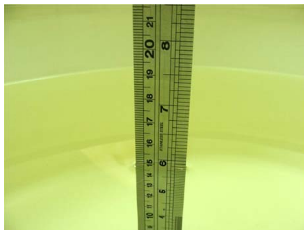
Fig 6.2 Photo of Liquid Height for Body SAR
