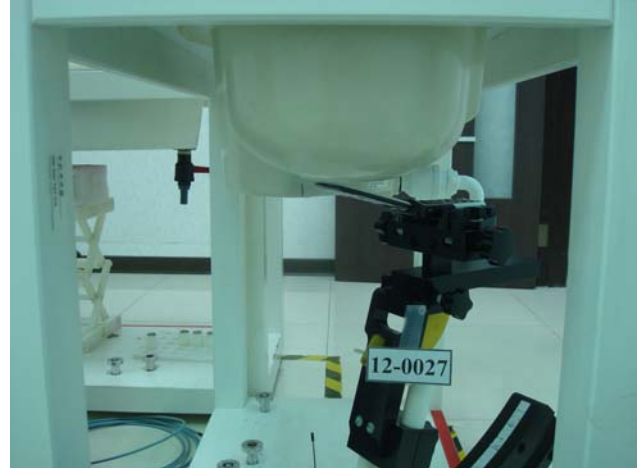
Figure 2. Right Head SAR Test Setup (Tilted)
