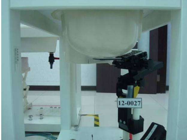
Figure 1. Right Head SAR Test Setup (Cheek)
