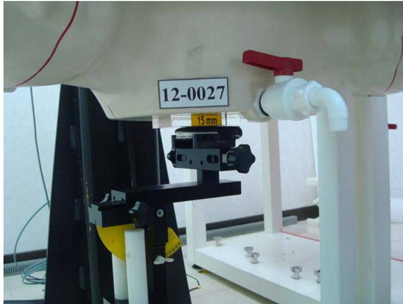
Figure 10. Body SAR Test Setup (Flat Section) _ Back Surface
