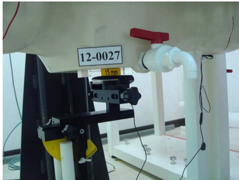
Figure 8. Body SAR Test Setup (Flat Section) _ Back Surface
