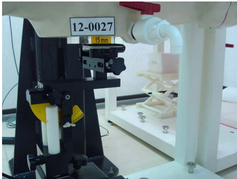
Figure 9. Body SAR Test Setup (Flat Section) _ Front Surface
