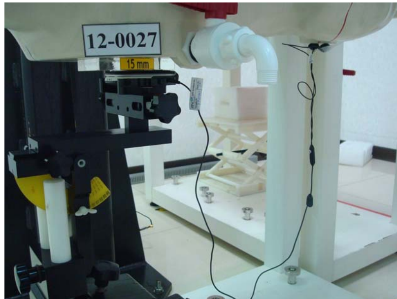
Figure 7. Body SAR Test Setup (Flat Section) _ Front Surface
