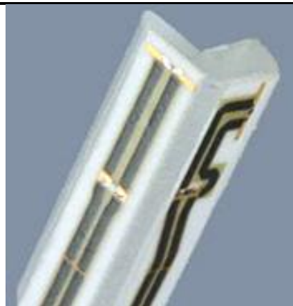
Fig. 5.2 Photo of E-field Probe
