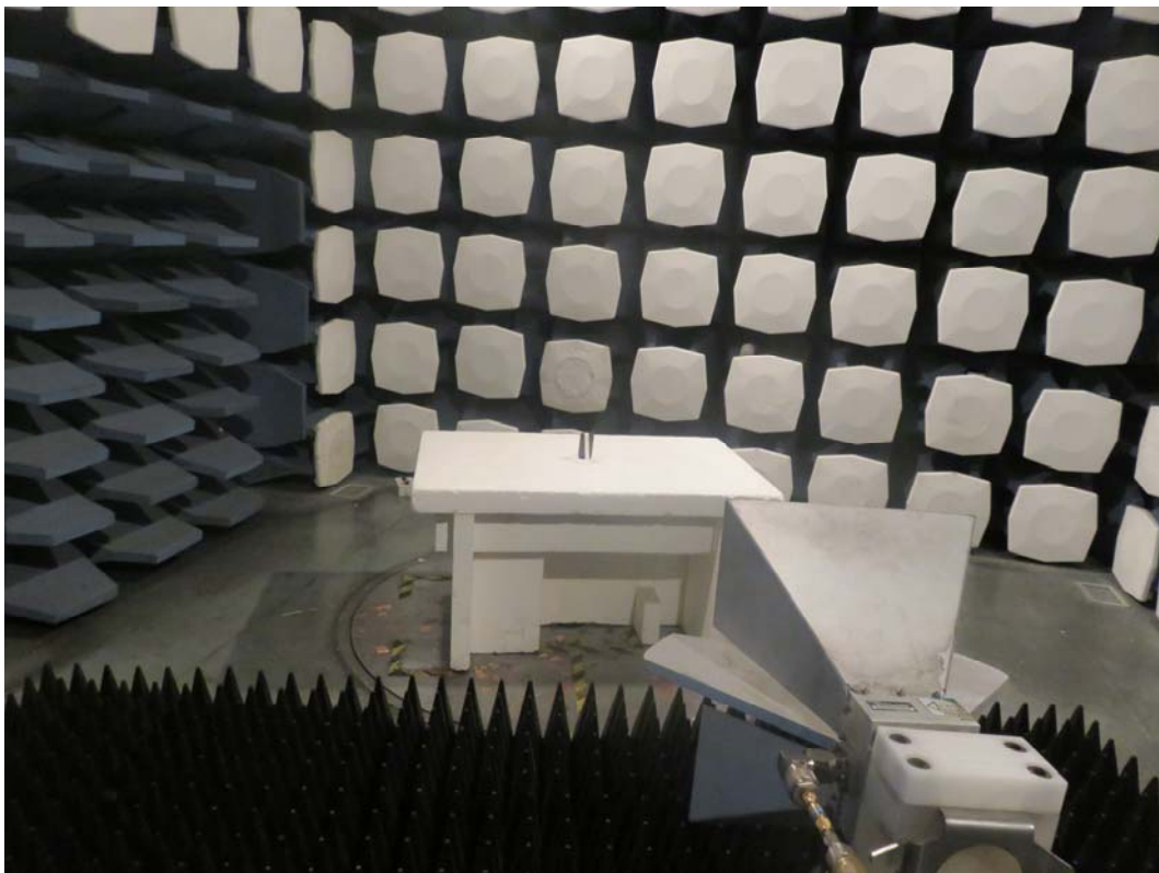
Picture 2: Radiated Spurious Emissions Test setup
