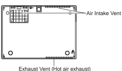
Exhaust Vent (Hot air exhaust)
