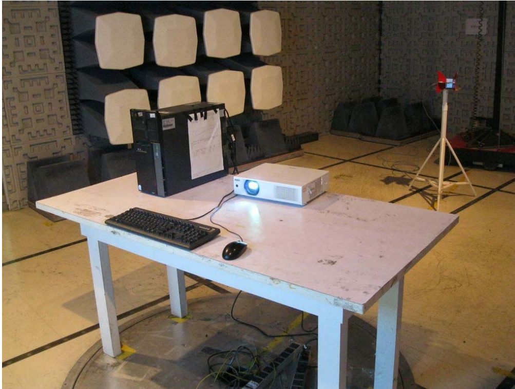
RADIATED EMISSION TEST SETUP (ABOVE 1G)
