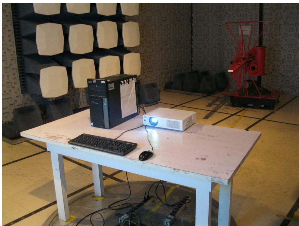
RADIATED EMISSION TEST SETUP (BELOW 1G)
