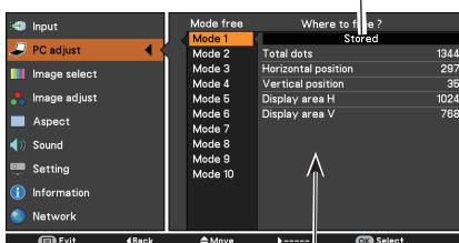
Values of Total dots, Horizontal position, Vertical position, Display area H, and Display area V.
