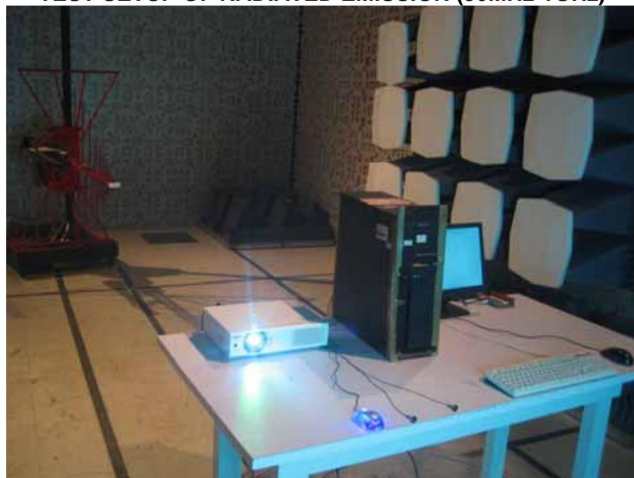
**TEST SETUP OF RADIATED EMISSION (above 1GHz)**
