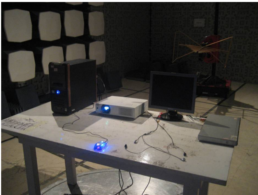
TEST SETUP OF RADIATED EMISSION (30MHz-1GHz)
