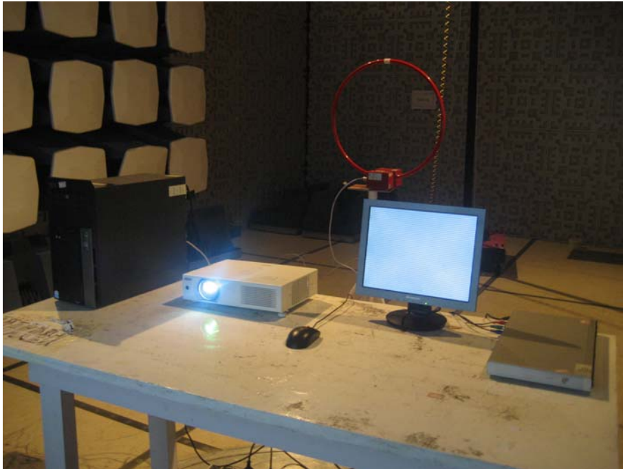
TEST SETUP OF RADIATED EMISSION (9kHz-30MHz)
