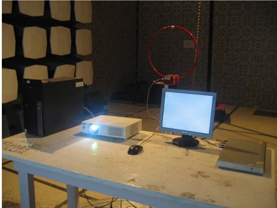
TEST SETUP OF RADIATED EMISSION (9kHz-30MHz)
