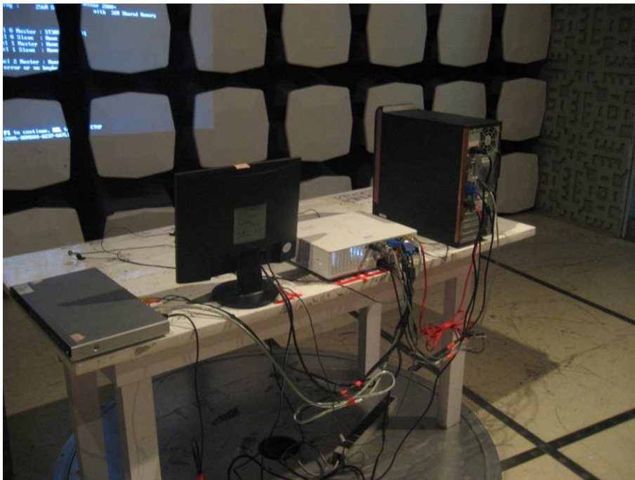
TEST SETUP OF RADIATED EMISSION - BACK VIEW
