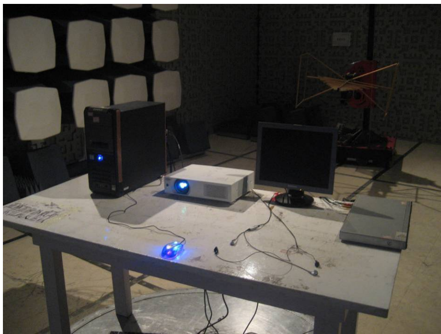
TEST SETUP OF RADIATED EMISSION (30MHz-1GHz)
