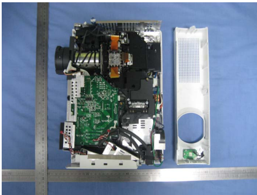
Internal View-2 (PCB 2 (left) & PCB 3 (right) in EUT)
