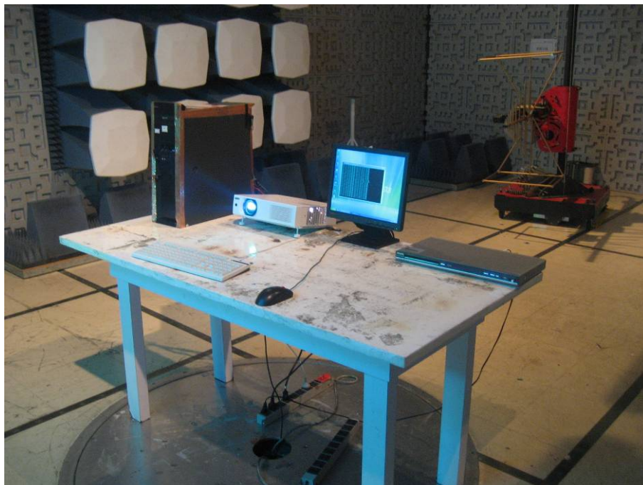
TEST SETUP OF RADIATED EMISSION (30MHz-1GHz)
