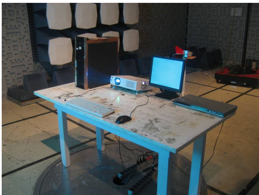
TEST SETUP OF RADIATED EMISSION (above 1GHz)
