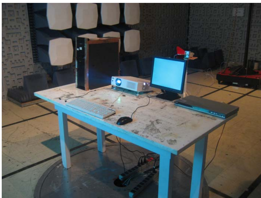
TEST SETUP OF RADIATED EMISSION (above 1GHz)
