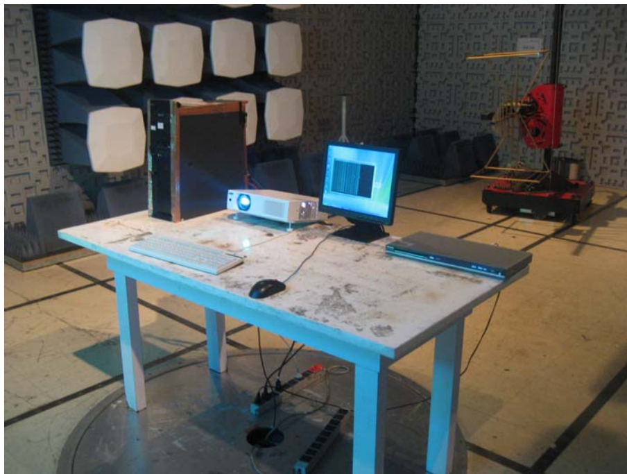
TEST SETUP OF RADIATED EMISSION (30MHz-1GHz)
