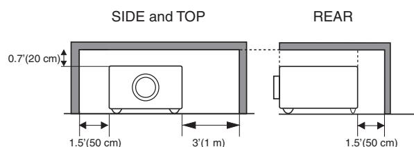
Do not cover the ventilation slot on the projector. Heat build-up can reduce the service life of your projector, and can also be dangerous.
