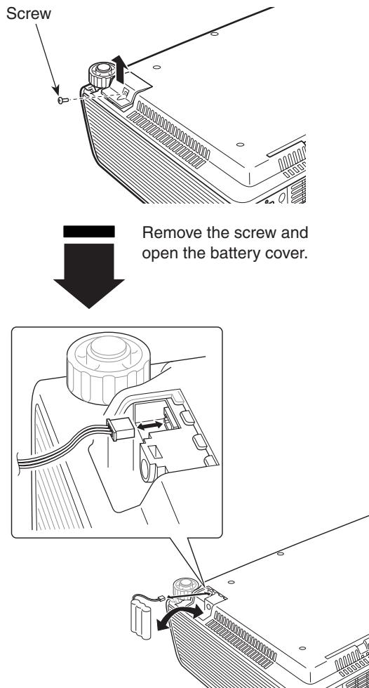
Install the battery, then put back the battery cover and secure it with the screw.
