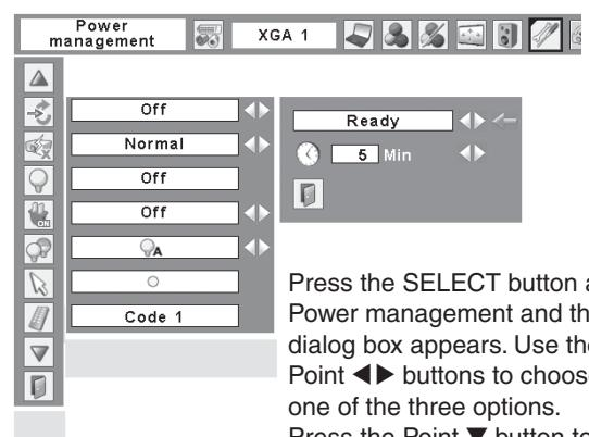
Press the SELECT button at Power management and this dialog box appears. Use the Point **◀▶** buttons to choose one of the three options. Press the Point **▼** button to select the timer, and then use the Point **◀▶** buttons to set timer.
