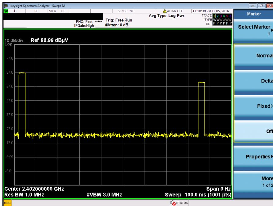
$$20\log(\text{Dwell Time}/100\text{ms}) = 20\log(\text{Time On} * \text{Number of hopping}/100\text{ms})$$
