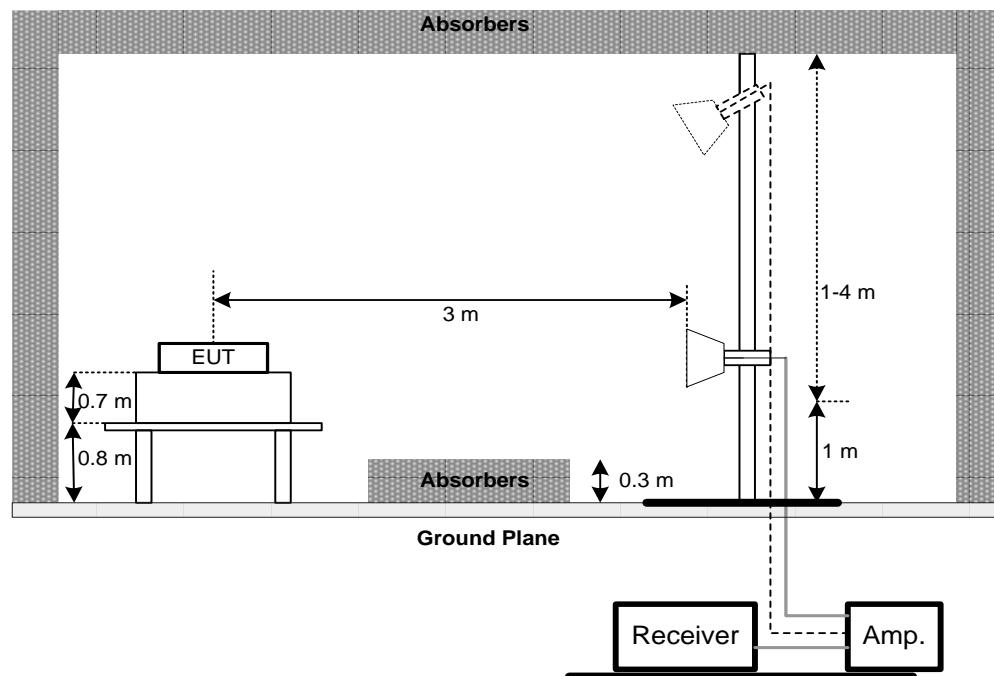
(C) For Radiated Emissions Below 30MHz
