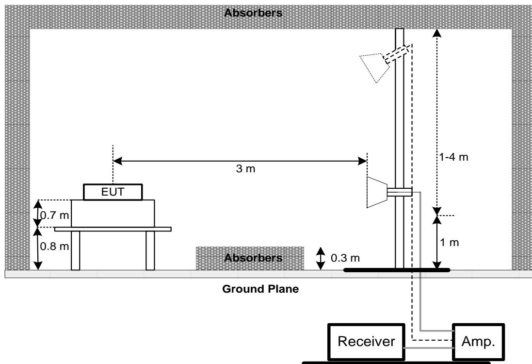
(C) For Radiated Emissions Below 30MHz
