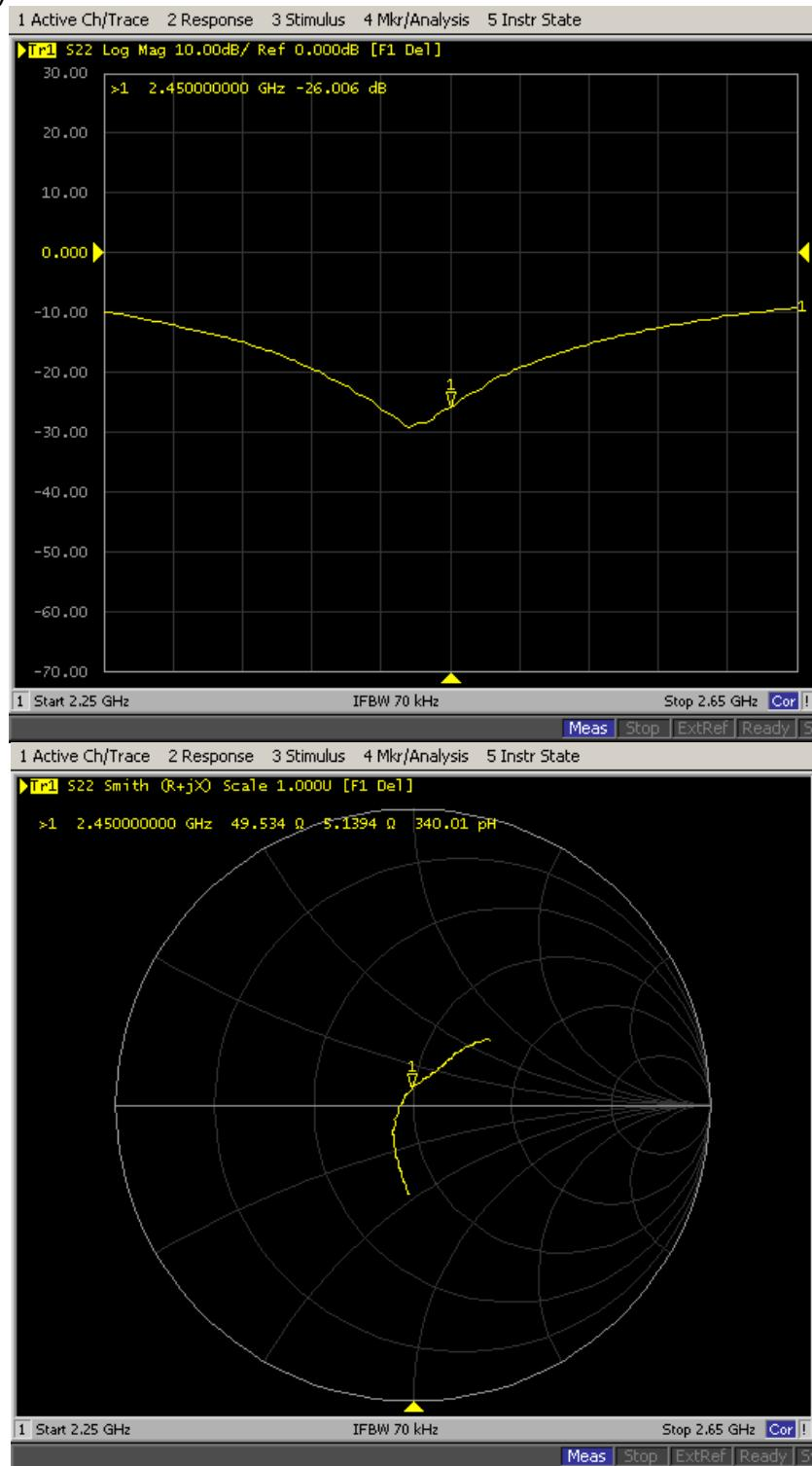
**D2450V2, Serial No.817 Extended Dipole Calibrations**
