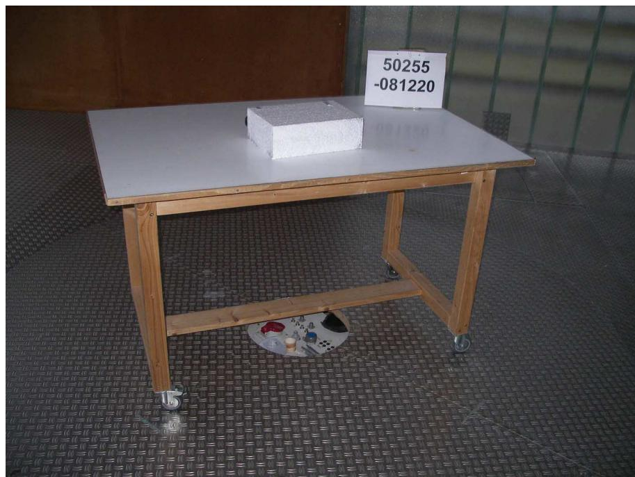
**Test setup for radiated emission measurement
