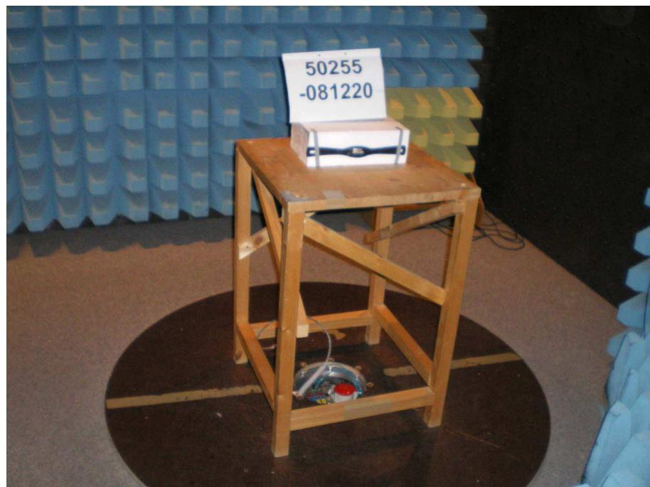
**Test setup for radiated emission measurement
