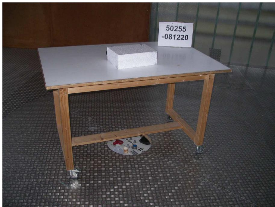
**Test setup for radiated emission measurement
