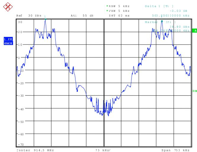
113961\_111.wmf: Channel separation at the upper end of the assigned frequency band:
