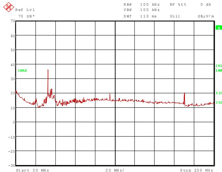
**113961\_62.wmf: Spurious emissions from 230 MHz to 1 GHz (operation mode 3, carrier notched):**
