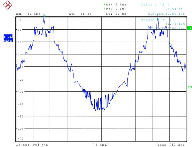
113961\_110.wmf: Channel separation at the middle of the assigned frequency band:
