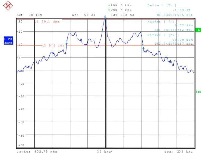
113961\_106.wmf: 20 dB bandwidth at the middle of the assigned frequency band:
