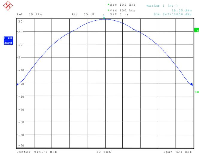
113961\_112.wmf: Maximum peak output power at the upper end of the assigned frequency band:
