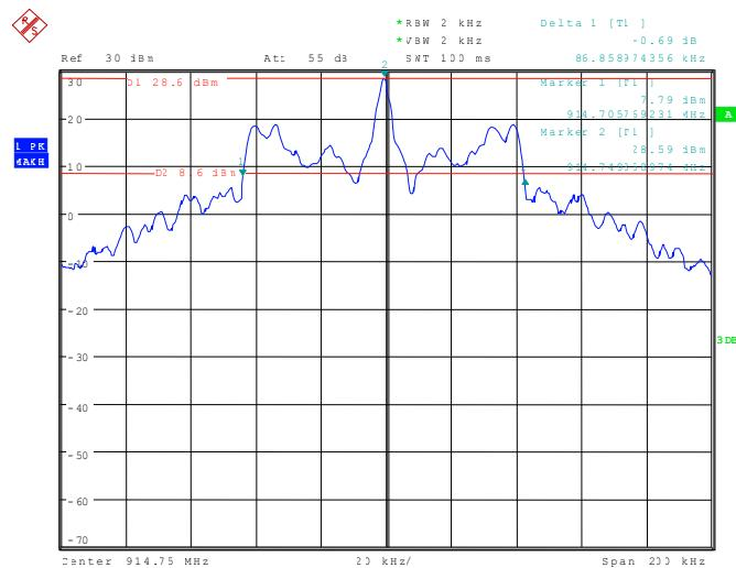
113961\_108.wmf: 20 dB bandwidth at the upper end of the assigned frequency band:
