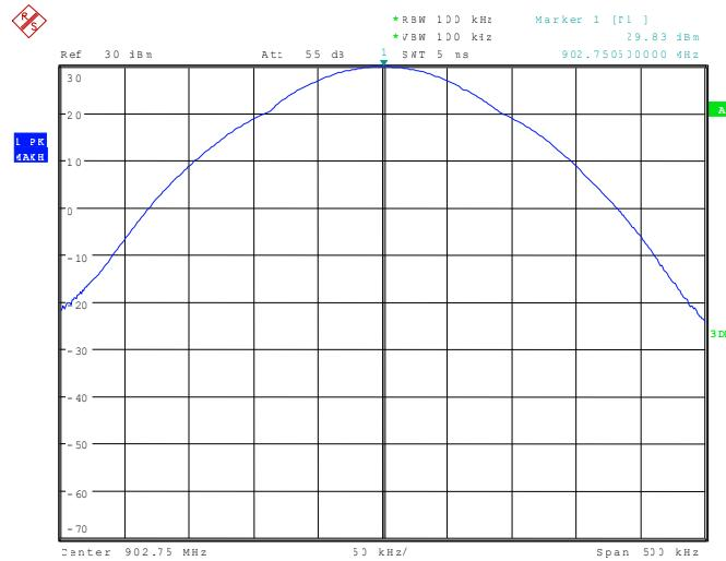
113961\_113.wmf: Maximum peak output power at the middle of the assigned frequency band:
