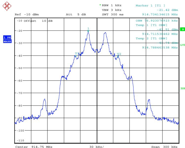
181673\_114.wmf: 99 % bandwidth at the upper end of the assigned frequency band:
