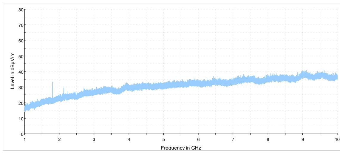
The following frequency was found outside the restricted bands during the preliminary radiated emission test:
