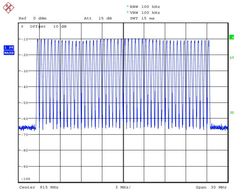
Remark: The Resolution bandwidth was set close to the 20 dB bandwidth in order to reach a better optical identification of the signal peaks.
