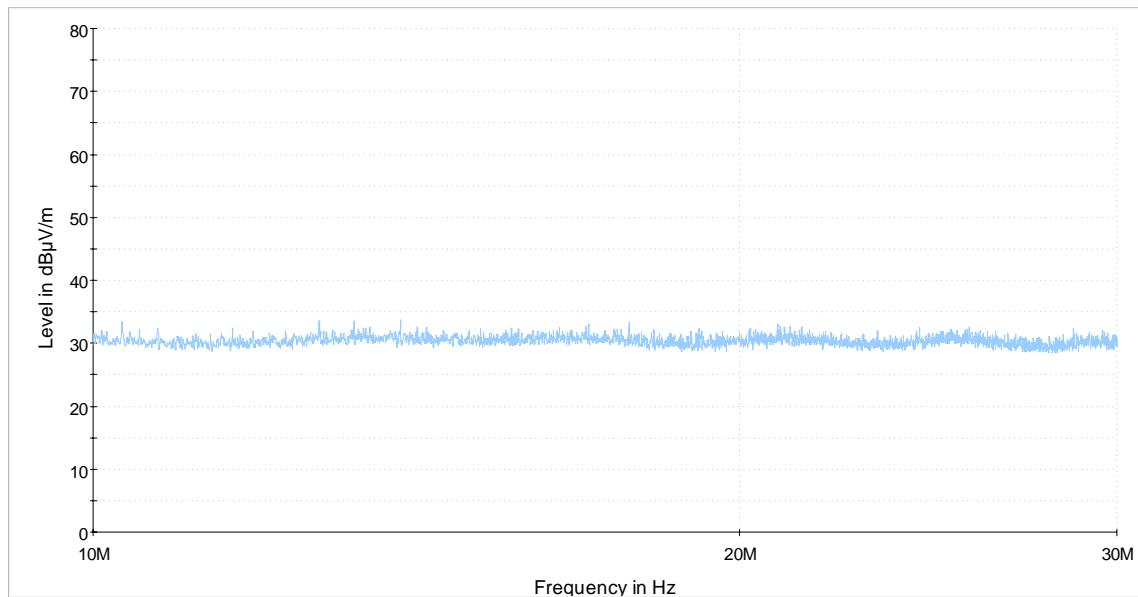
No significant frequencies above the noise floor of the system (max. 34 dB $\mu$ V/m (measured with peak detector) at 3 m distance) were found during the preliminary radiated emission test, so no measurements were carried out on the outdoor test site.
