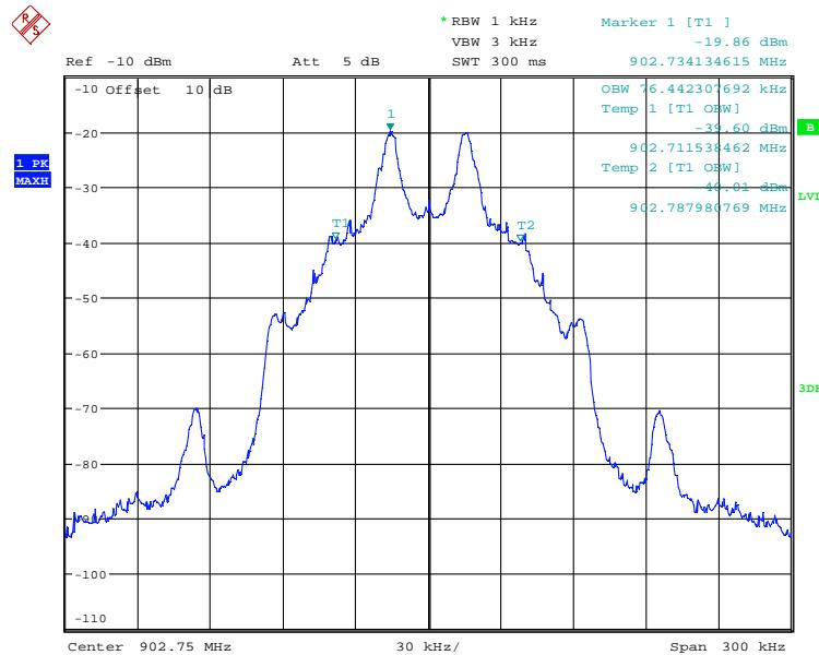
181673\_113.wmf: 99 % bandwidth at the middle of the assigned frequency band:
