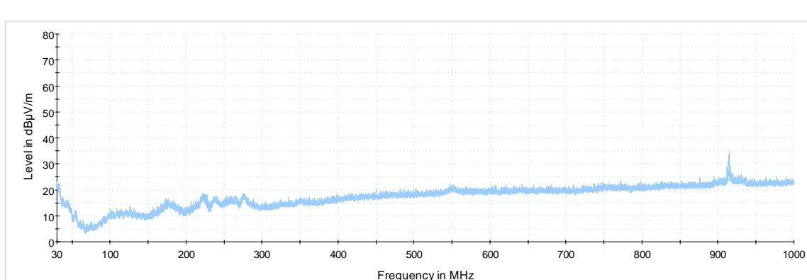
The following frequencies were found outside the restricted bands during the preliminary radiated emission test:
