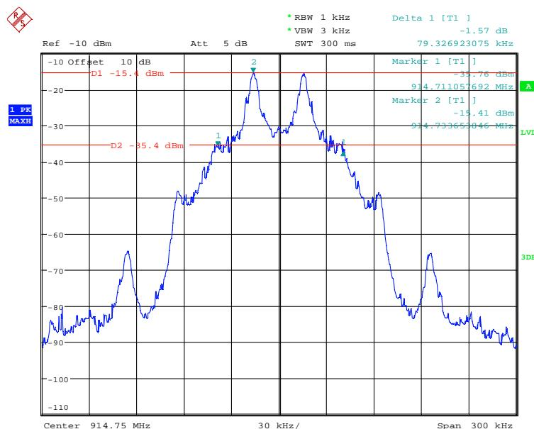
181673\_103.wmf: 20 dB bandwidth at the upper end of the assigned frequency band:
