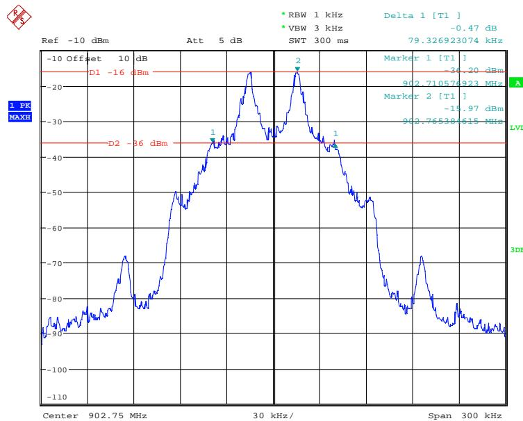
181673\_102.wmf: 20 dB bandwidth at the middle of the assigned frequency band:
