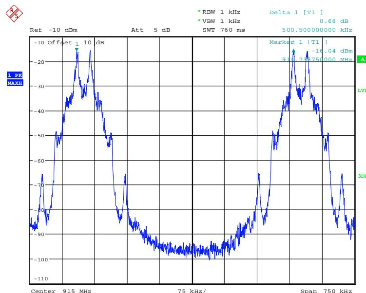
181673 .wmf: Channel separation at the upper end of the assigned frequency band:
