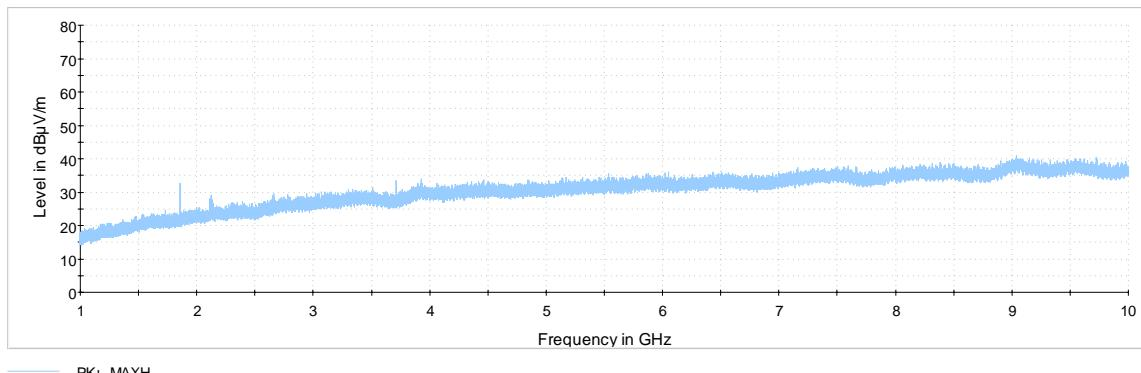
The following frequencies were found outside the restricted bands during the preliminary radiated emission test:
