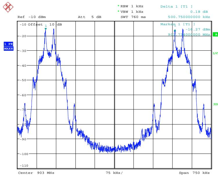
181673\_105.wmf: Channel separation at the middle of the assigned frequency band:
