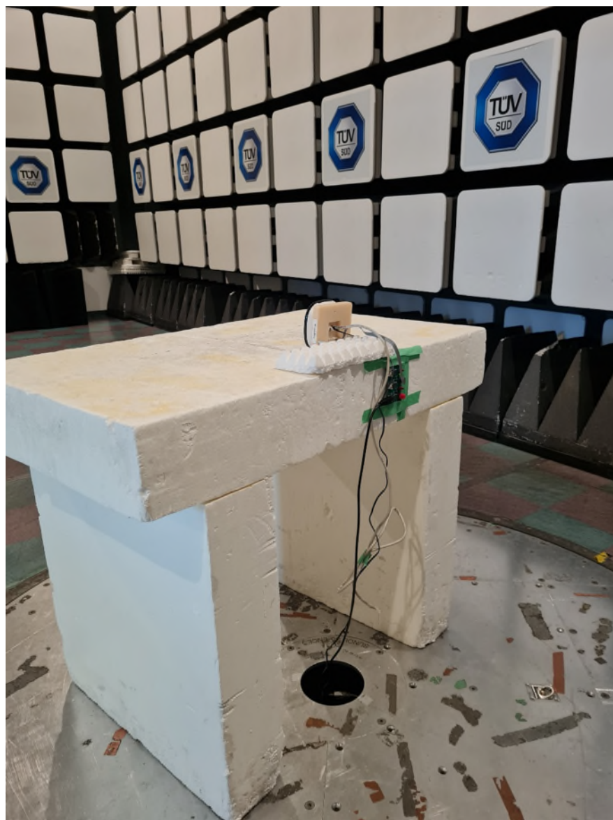
Figure 1 – Radiated Emissions Setup
