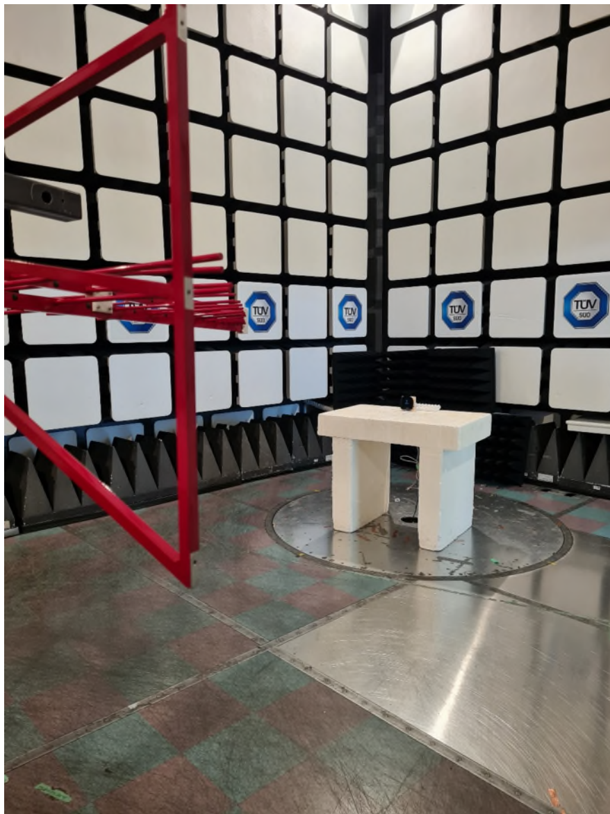
Figure 3 – Radiated Emissions Setup 30MHz – 1GHz
