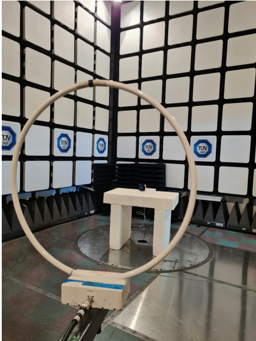
Figure 2 – Radiated Emissions Setup 9kHz – 30MHz
