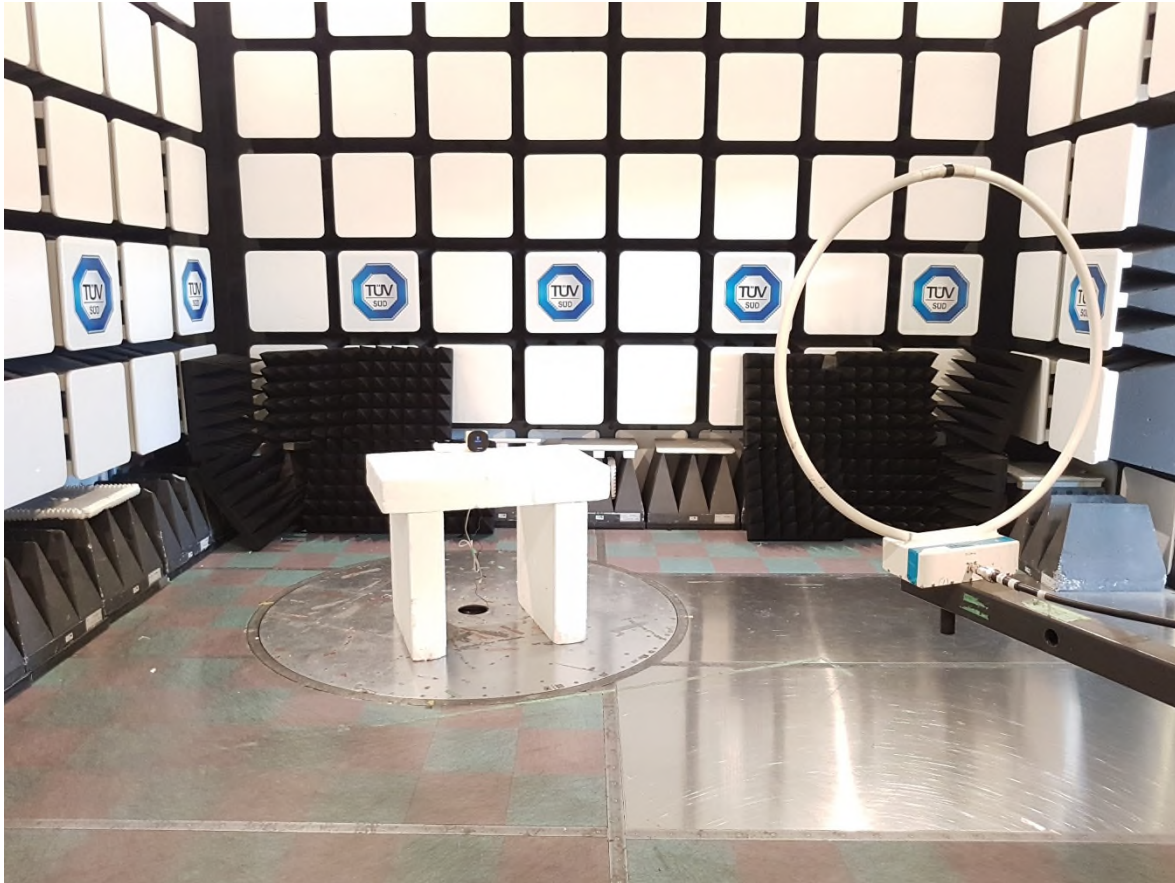
Figure 4 – Radiated Emissions Setup 9kHz – 30MHz
