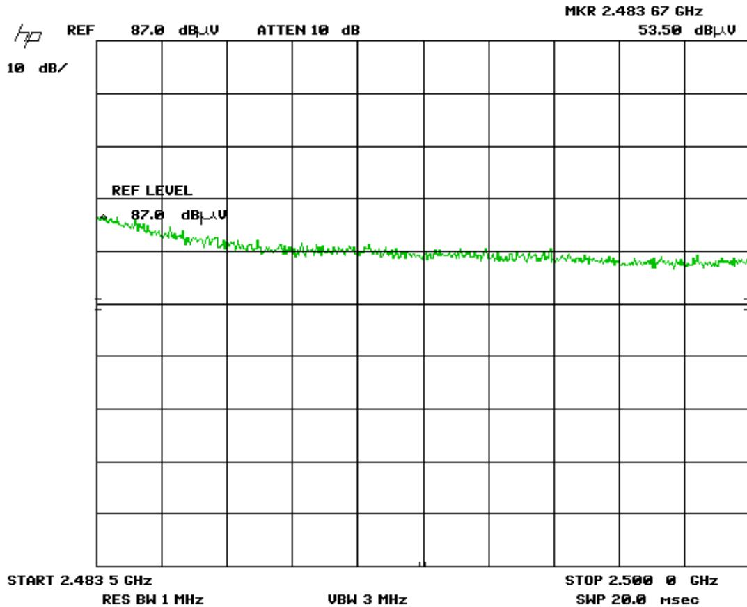
Note: Band edge plots were taken with 3 m measurements distance. The marker shows the raw value; see Final Measurements and Results section starting on page 72 for corrected values.
