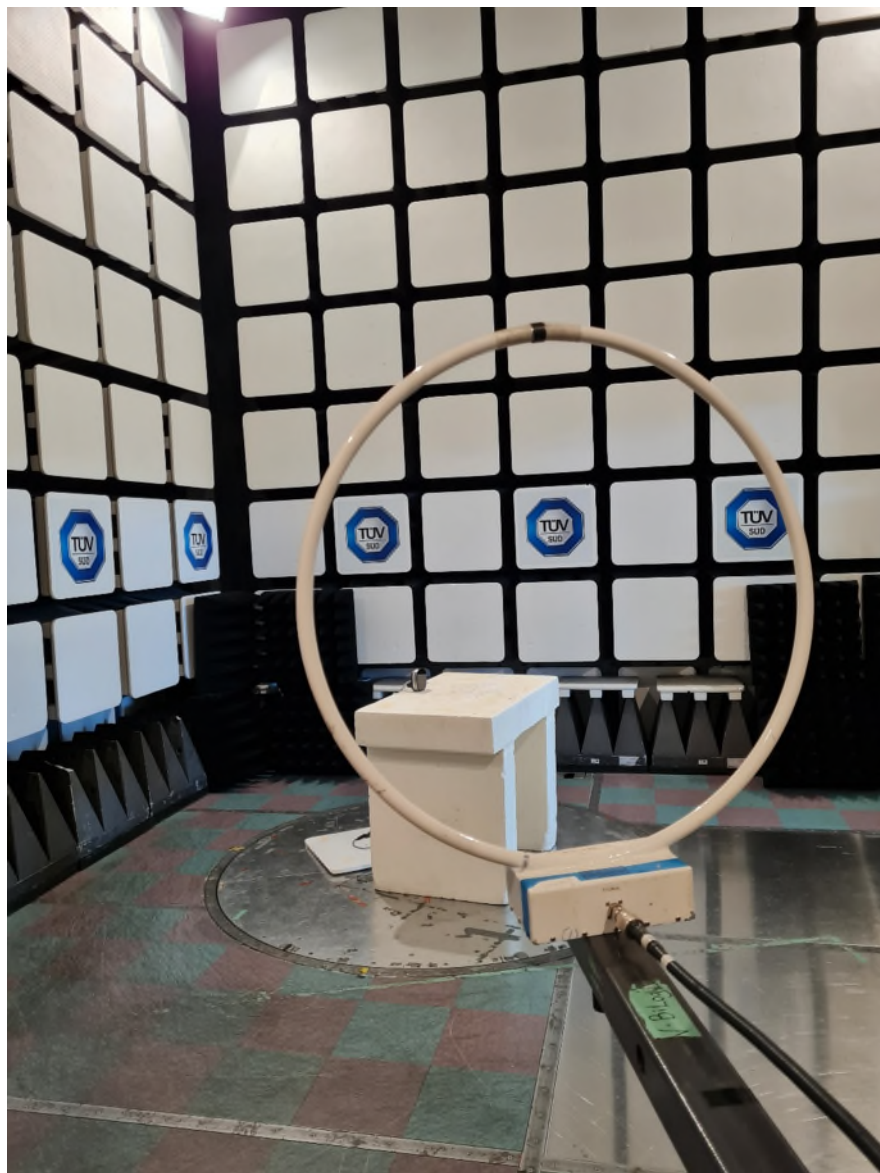
Figure 1 – Radiated Emissions Setup 9kHz – 30MHz
