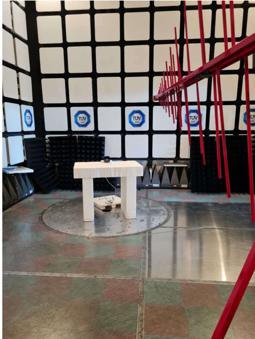
Figure 2 – Radiated Emissions Setup 30MHz – 1GHz
