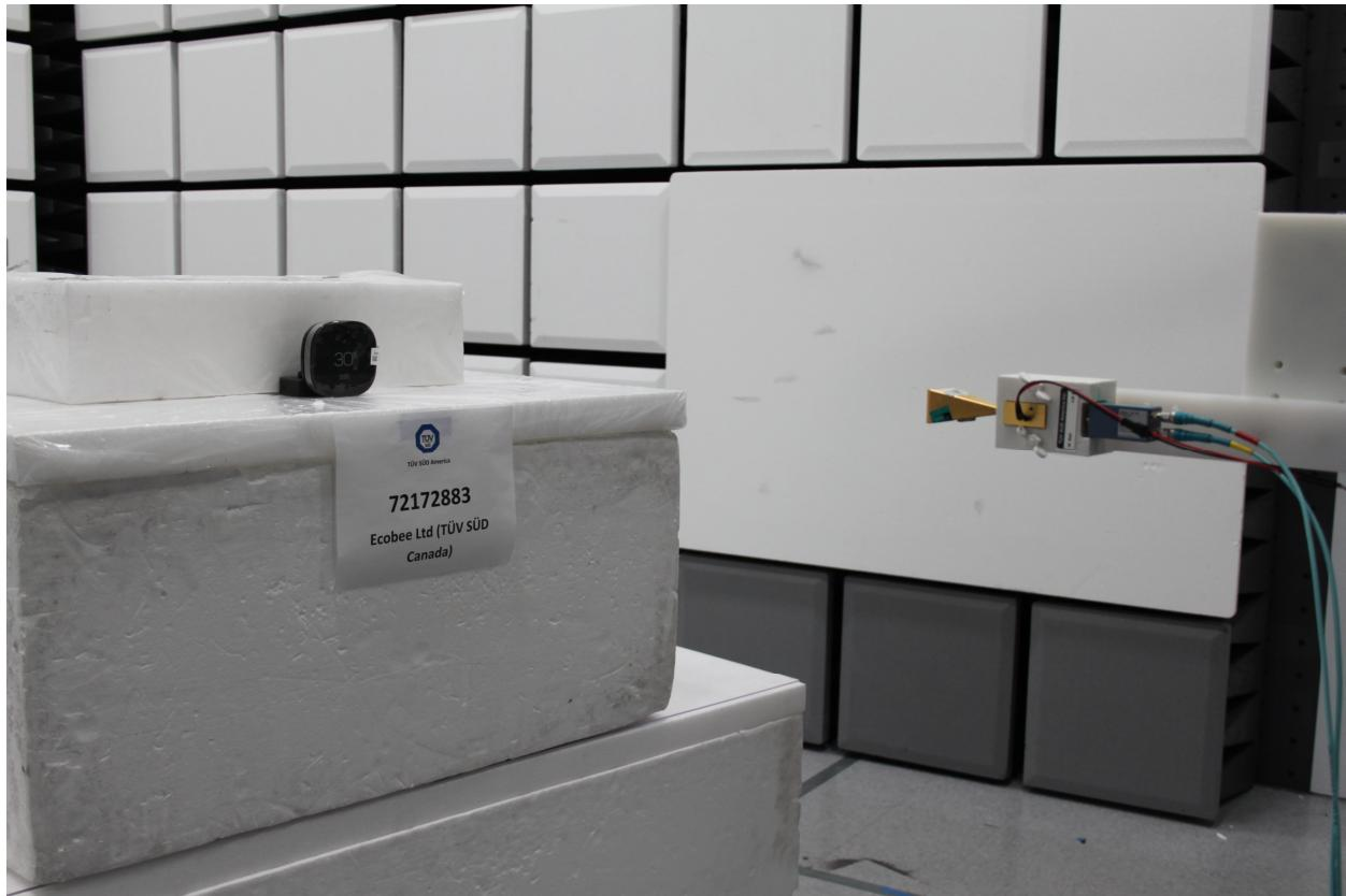
**Radiated Emissions Test Setup (40GHz to 100GHz)**
