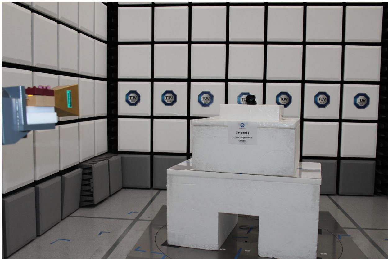
**Radiated Emissions Test Setup (18GHz TO 40GHz)**
