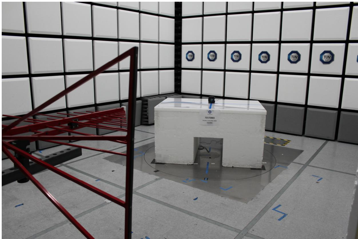
**Radiated Emissions Test Setup (30MHz to 1GHz)**
