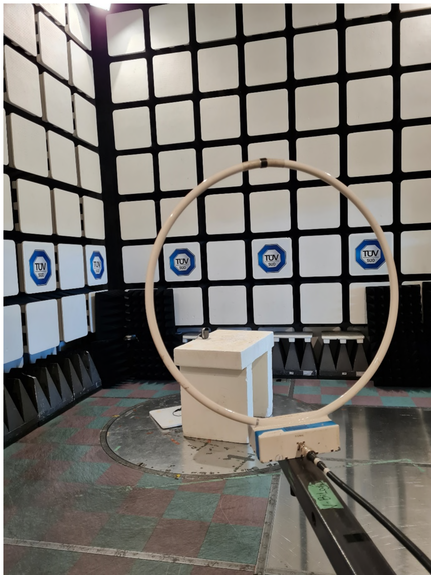
Figure 1 – Radiated Emissions Setup 9kHz – 30MHz
