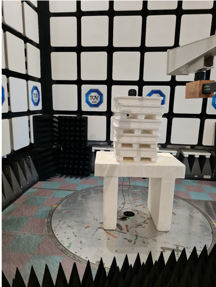
Figure 4 – Radiated Emissions Setup 1 > 1GHz
