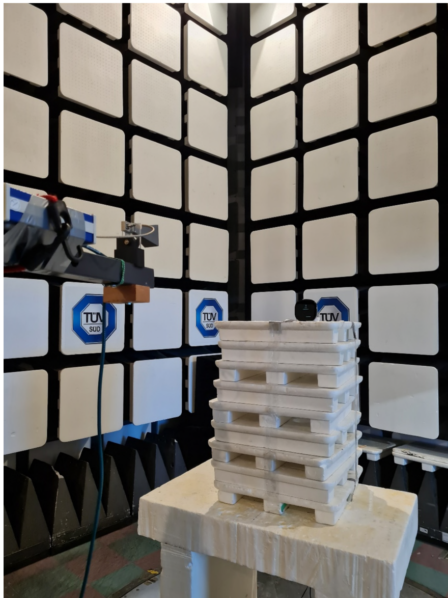
Figure 5 – Radiated Emissions Setup 1 > 1GHz
