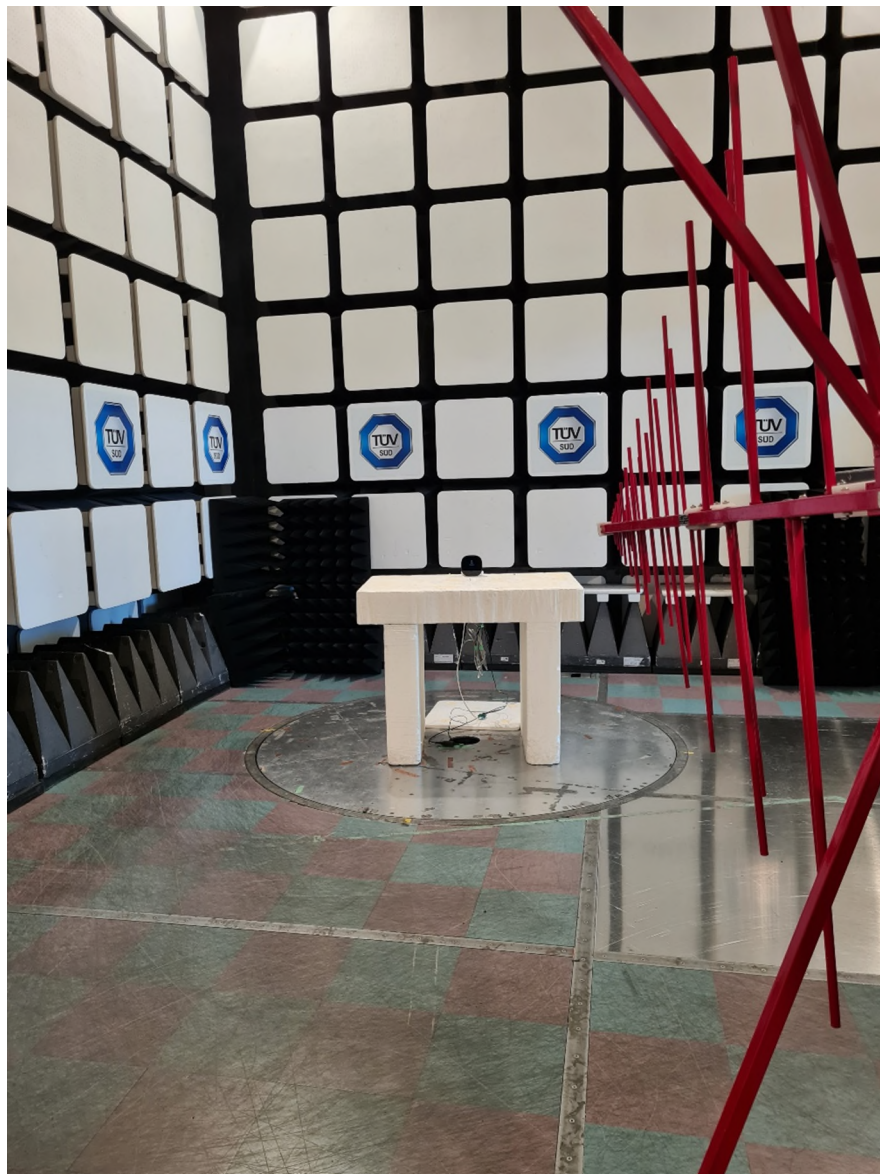
Figure 2 – Radiated Emissions Setup 30MHz – 1GHz
