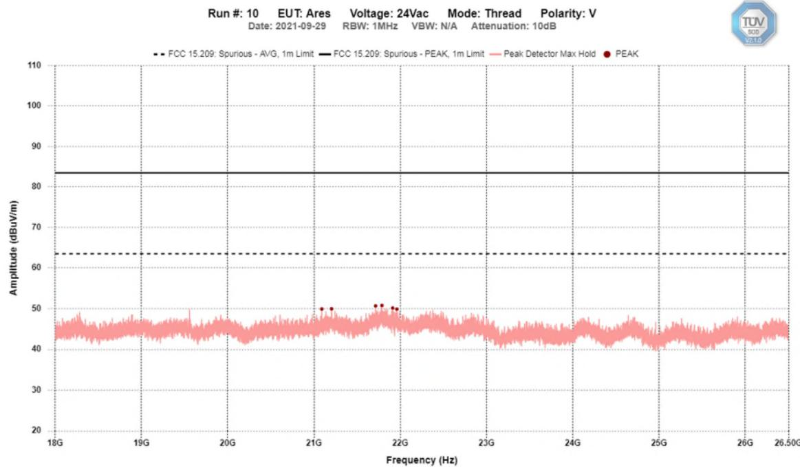
Plot was taken at a 1 meter distance. All emissions were noise floor of measurement instrument. No emissions were found in this frequency range.
