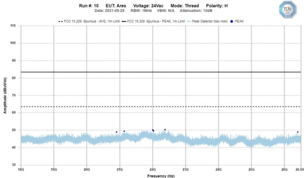
**Note: 12 GHz – 26 GHz plots were taken at a 1 meter distance. All emissions were noise floor of measurement instrument. No emissions were found in this frequency range.**
