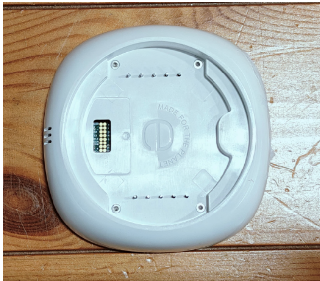
Figure 3 – Smart Thermostat Lite: Back view with I/O ports
