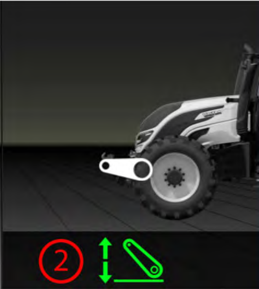
Indicates whether single acting or double acting mode is enabled.
