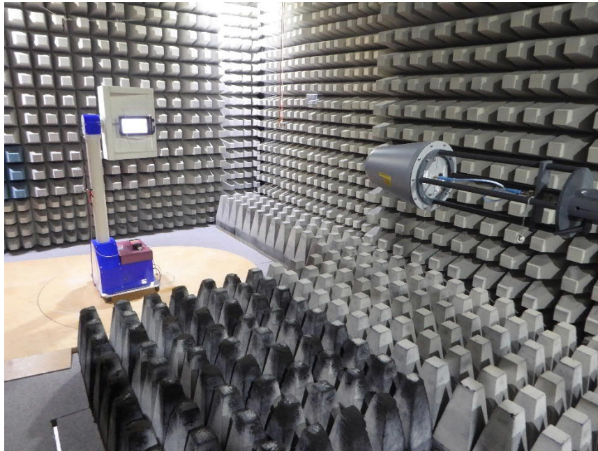
EUT on positioner Test setup fully anechoic chamber M20 Preliminary and final measurement 1 – 12 GHz
