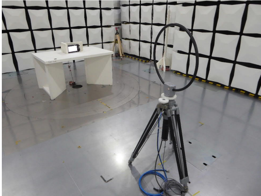
EUT Position 1 – standing / Antenna Position 2 – parallel Test setup semi-anechoic chamber M276 Preliminary measurement
