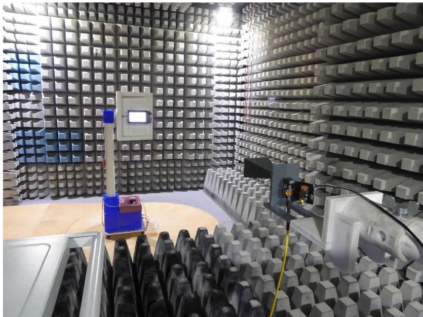
EUT on positioner Test setup fully anechoic chamber M20 Preliminary and final measurement 12 – 18 GHz
