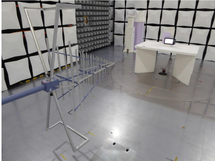
EUT Position 1 – standing Test setup semi-anechoic chamber M276 Preliminary and final measurement
