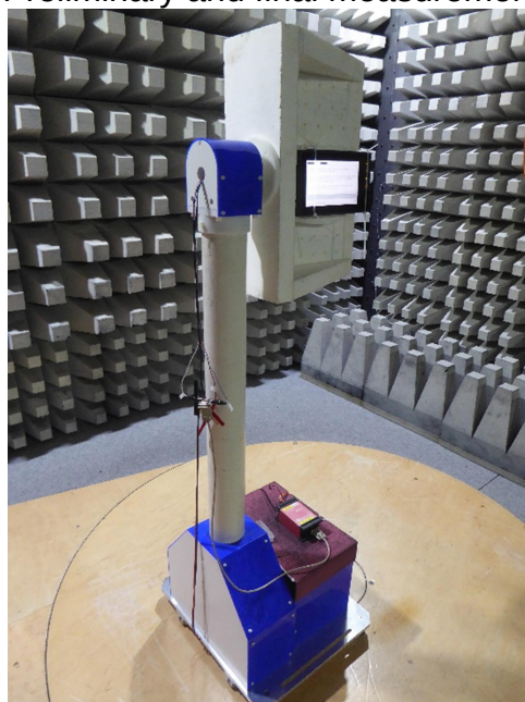
EUT on positioner Test setup fully anechoic chamber M20 Preliminary and final measurement
