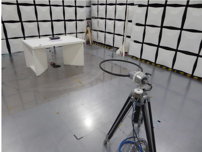
EUT Position 3 – lying / Antenna Position 3 – grund-parallel Test setup semi-anechoic chamber M276 Preliminary measurement
