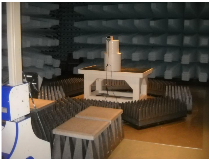
Set-up for radiated emission above 1 GHz
