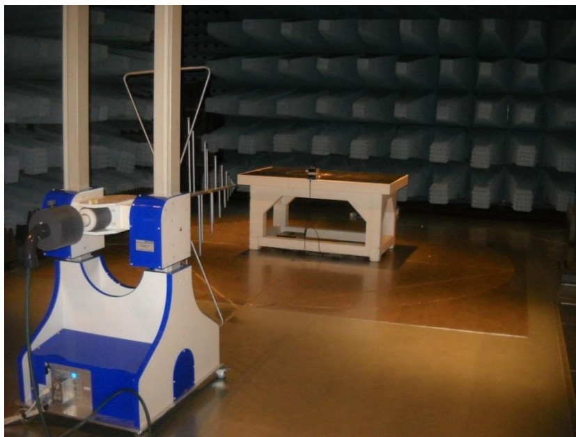
Set-up for radiated emission below 1 GHz
