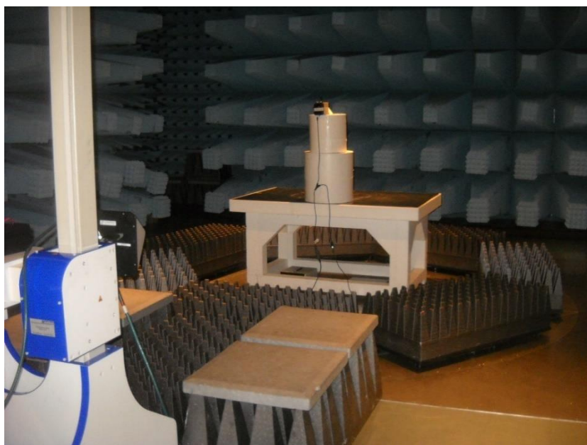
Set-up for radiated emission above 1 GHz
