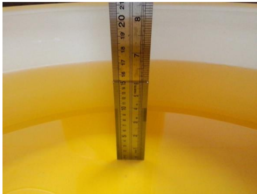
Photo 1: Tissue Simulant Liquid for Head 2300-2500
