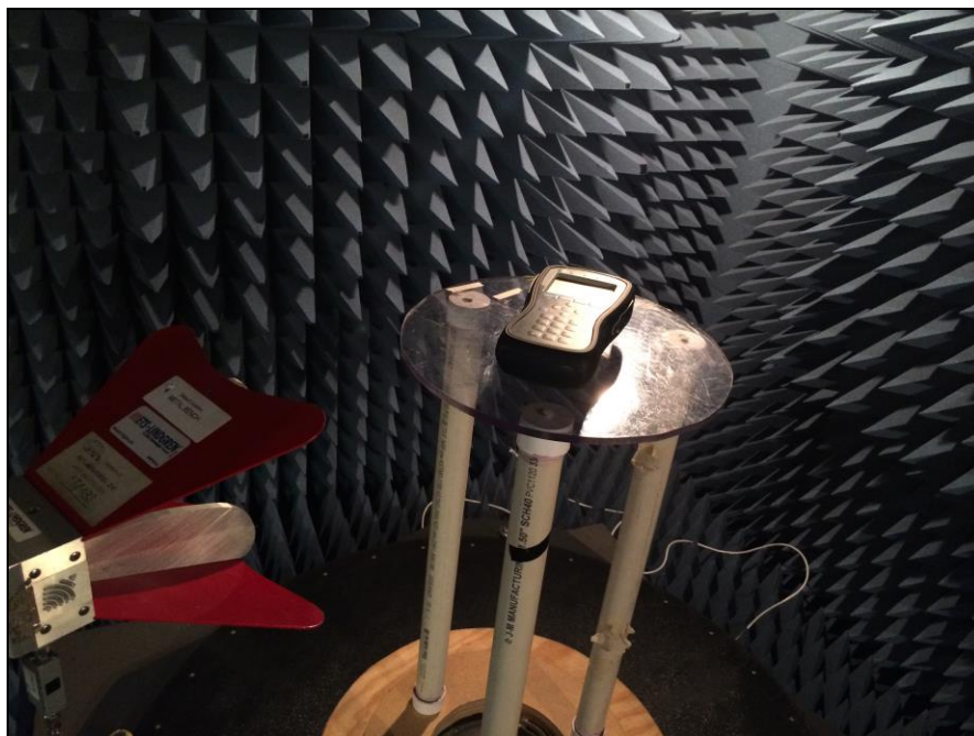
Photograph 7. Radiated Spurious Emissions, Test Setup, Above 1 GHz
