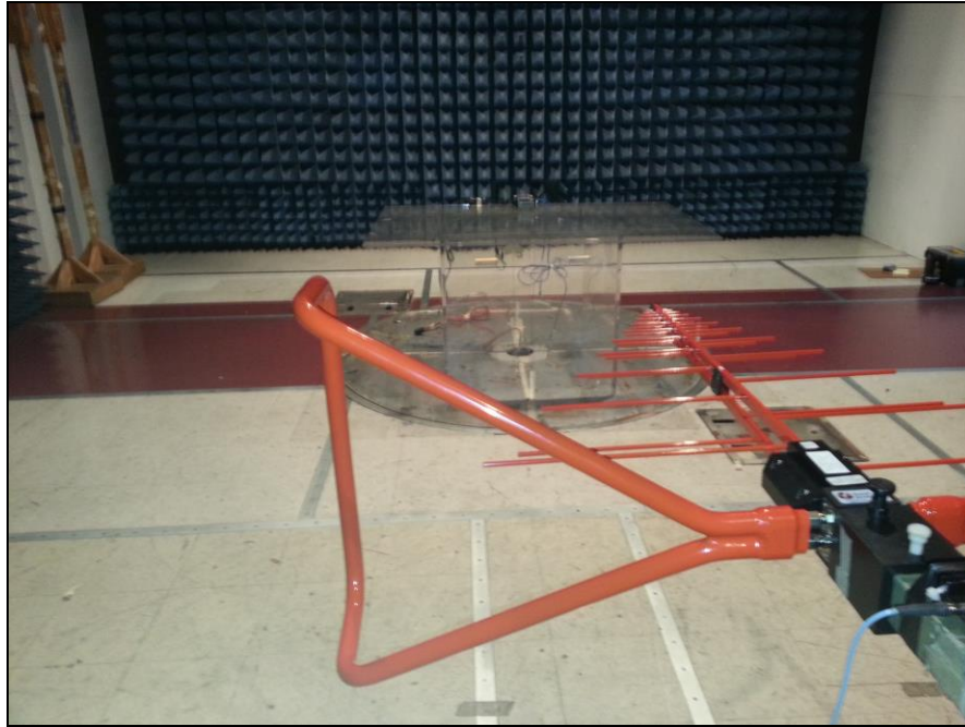
Photograph 3. Radiated Emissions, Test Setup, 30 MHz – 1 GHz
