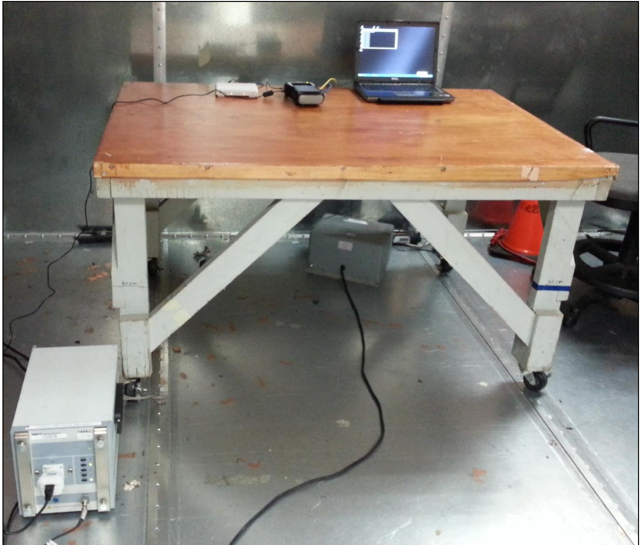
Photograph 5. Conducted Emissions, 15.207(a), Test Setup
